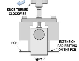
Move the extraction tool away from the printed circuit board.
