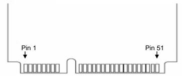
Figure 1-1 Apacer mSATA A1-M pin assignment
