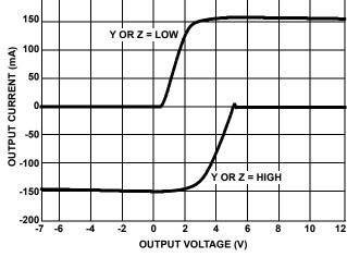
FIGURE 10. DRIVER OUTPUT CURRENT vs SHORT CIRCUIT VOLTAGE
