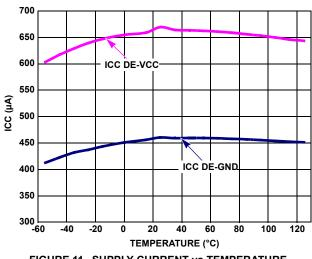
FIGURE 11. SUPPLY CURRENT vs TEMPERATURE
