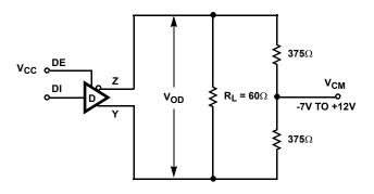
FIGURE 1B. VOD WITH COMMON MODE LOAD
