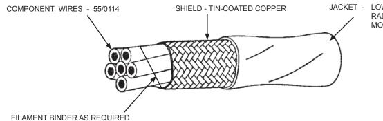
JACKET - LOW OUTGASSING, RADIATION-CROSSLINKED, MODIFIED ETFE
