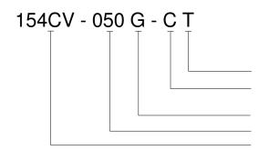
Vent (T = Tube, Blank = No Tube)
